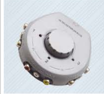
H14-005 3 way selector For transmission of analogue audio/video signal 3 x 3RCA input 1 x 3RCA output
