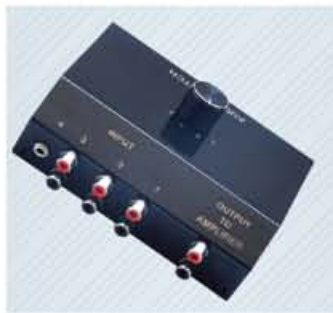
H14-012 3 way selector For transmission of analogue audio signal 3 x 2RCA input 1 x 2RCA output with 3.5mm stereo jack and switch
