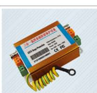
H20-040 CCTV surge protection Video protection=75Ω Data: RS485 Power: 220V Isn=5KA Imax=10KA
